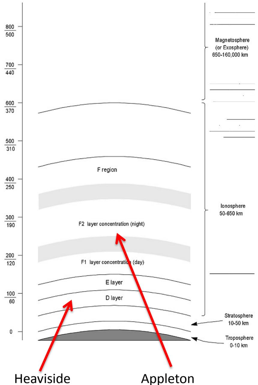
The lowest is D-layer at altitudes ranging from 50 to 90 km. High frequencies (3-30 MHz) penetrate this layer, while low frequency (LF: 30-300 kHz) or medium waves are absorbed by this layer. To some extent LF and Very Low Frequency (VLF: 3 to 30 kHz) are reflected during daytime. It slightly scatter and absorbs HF. This layer subsists only during daytime
