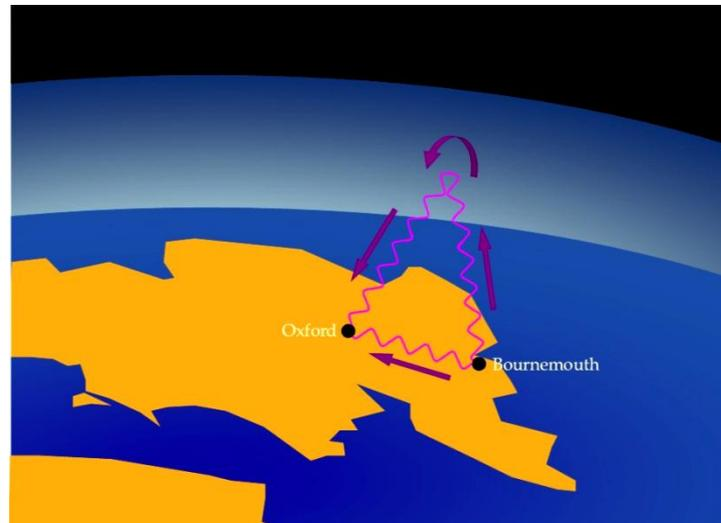
In 1924 Appleton was able to demonstrate the existence of the electrified reflecting layer in the upper atmosphere.
