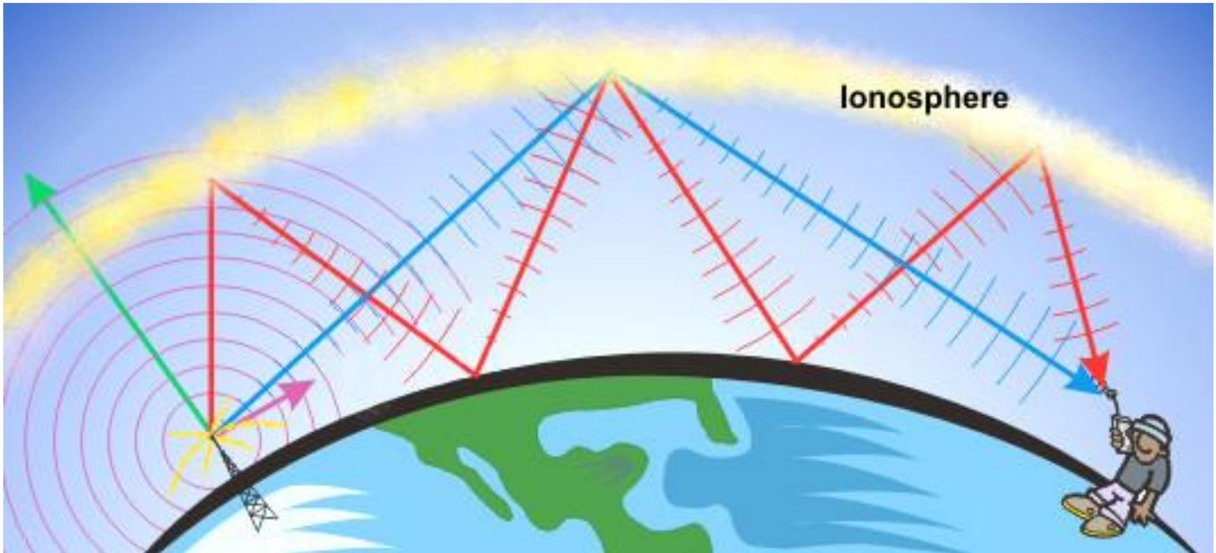
Further experiments which led to the possibility of round-the-world broadcasting were carried out and in 1926 he discovered a further atmospheric layer 150 miles above ground, higher than the Heaviside Layer and electrically stronger. This layer, named the Appleton Layer after him, reflects short waves round the earth.
