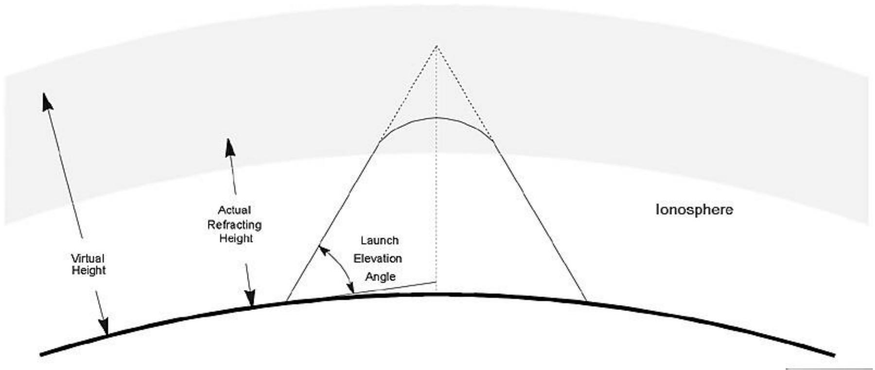
**Gradual refraction in the ionosphere allows radio signals to be propagated long distances. It is often convenient to imagine the process as a reflection with an imaginary reflection point at some virtual height above the actual refracting region.**
