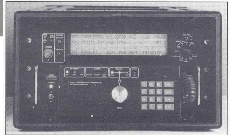
Figure 2. An ionosonde transmitter. Photo courtesy Gerald Oicles/BR Communications, Sunnyvale, CA
